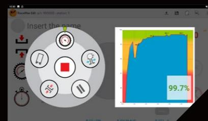
The chart realized in real time allows for immediate visual feedback about the quality of the vacuum in the mold, an essential phase for the success of the injection.
