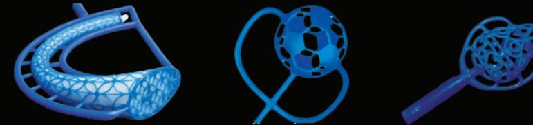
Sensitive to all market requests, Riacetech has developed a wax injection process based on hydro soluble support. It will be possible to realize 3D filigreed and hollow objects using normal wax and soluble material.
